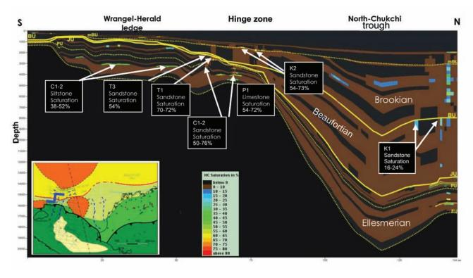
**Fig. 3.** Present-day hydrocarbon saturation across the North Chukchi basin (south to north cross-section – TemisSuite basin modeling)
